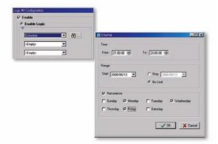
is useful when applied to energy savings, lighting control, and water pumping systems. The timer function allows users to set a delay period for actions, which is particularly useful when used with alarm systems for which users need an authentication period to avoid false alarms.
